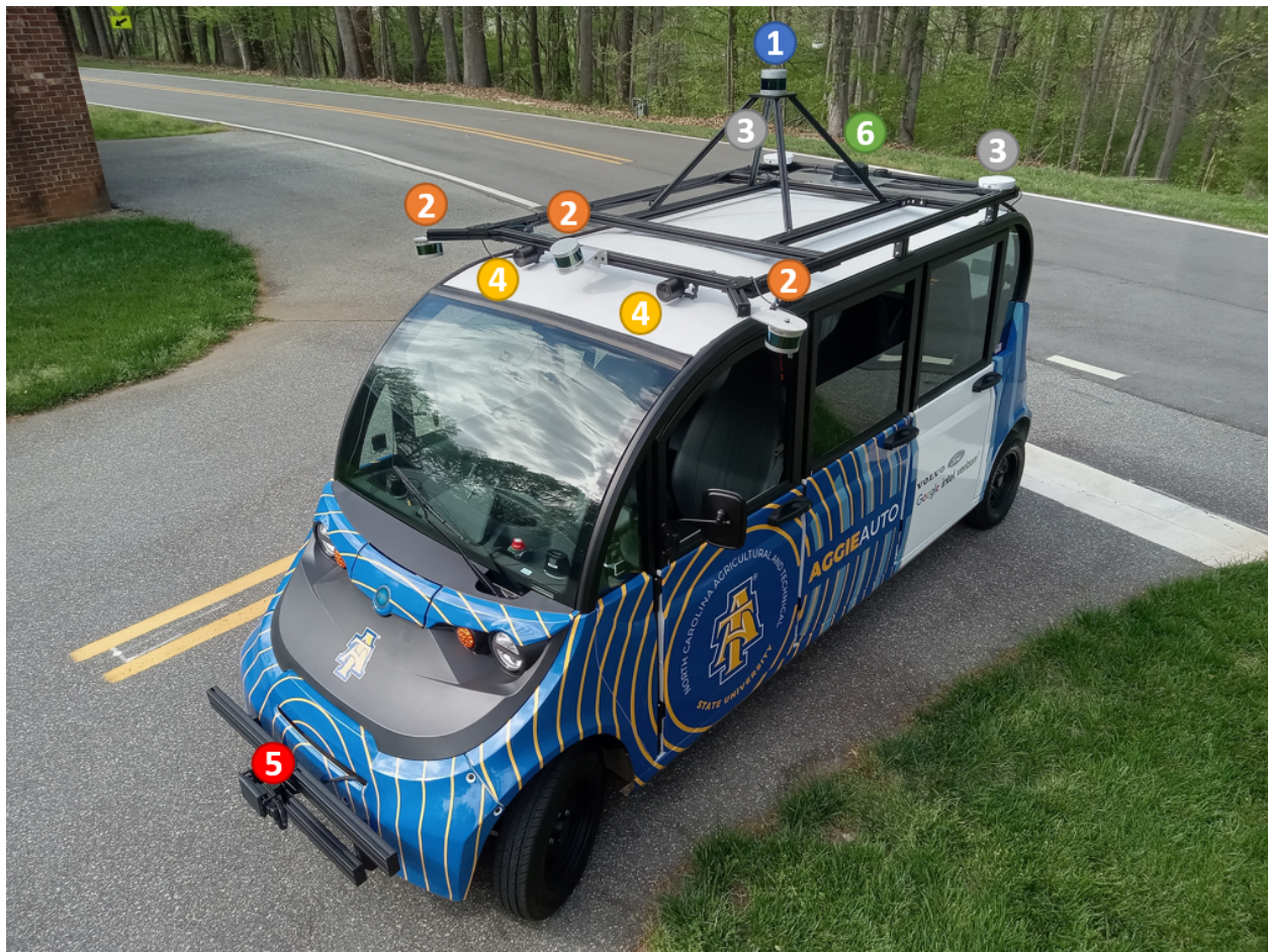
Figure 1. Sensor suite consisting of: 1) Velodyne VLP-32C, 2) 3x Velodyne VLP-16, 3) Dual Antenna + Novatel PwrPak7D-E2, 4) 2x Lucid Triton Camera IMX265, 5) RaDAR Delphi ESR, and 6) MAKO 5G Dome Antenna + Cradlepoint R1900.
